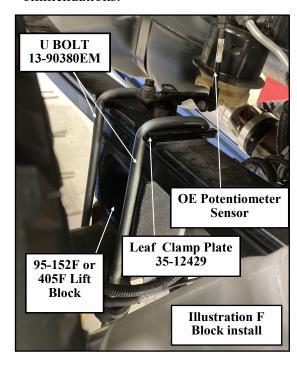
16. Torque all bolts to factory specifications. Re-torque all bolts after 500 miles.
